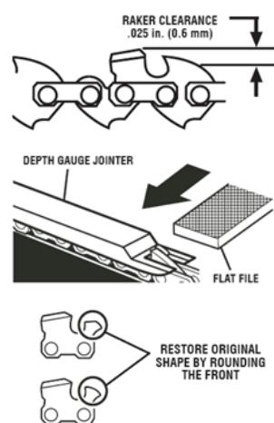
Every time the chain is filed, check the depth gauge clearance
