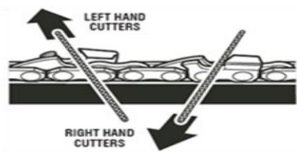
Put a few firm strokes on every tooth. File all left hand cutters in one direction. Then move to the other side and file the right hand cutters in the opposite direction. Occasionally remove filing from the file with a wire brush.
