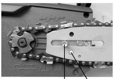
VIS DE GUIDAGE      VIS DE TENSION
