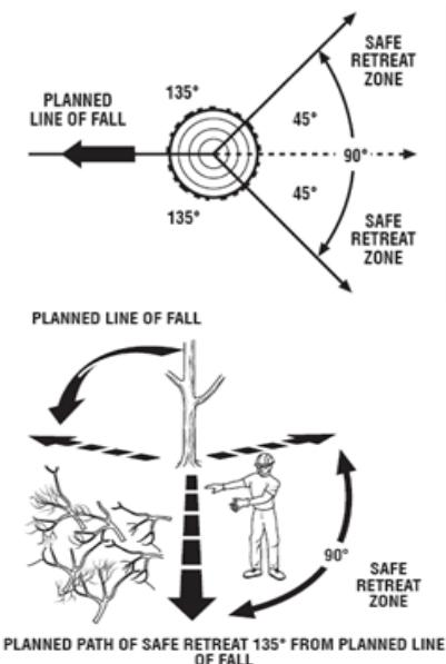
Before felling is started, consider the force and direction of the wind, the lean and balance of the tree, and the location of large limbs. These things influence the direction in which the tree will fall. Do not try to fell a tree along a line different from its natural line of fall.
