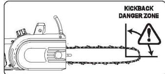
**WARNING:** Do Not use the chain saw with any type of accessory or attachment. Such usage might be hazardous.
