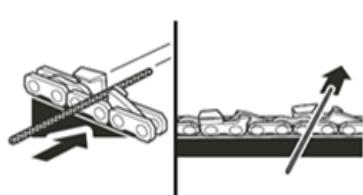
Lift file away from the steel on each return stroke.
