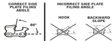
Hook – "Grabs" and dulls quickly. Increases potential of kickback. Results from using a file with a diameter too small, or file held too low.
