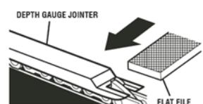
Depth gauges must be adjusted with the flat file in the same direction the adjoining cutter was filed with the round file. Use care not to contact cutter face with flat file when adjusting depth gauges.
