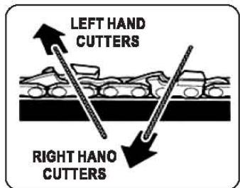
**WARNING:** Improper chain sharpening increases the potential of kickback.
