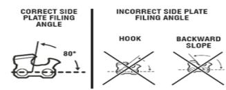
Backward Slope – Needs too much feed pressure, causes excessive wear to bar and chain. Results from using a file with a diameter too large, or file held too high.
