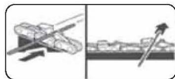
Lift file away from the steel on each return stroke.
