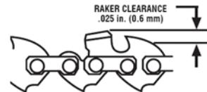
Every time the chain is filed, check the depth gauge clearance.
