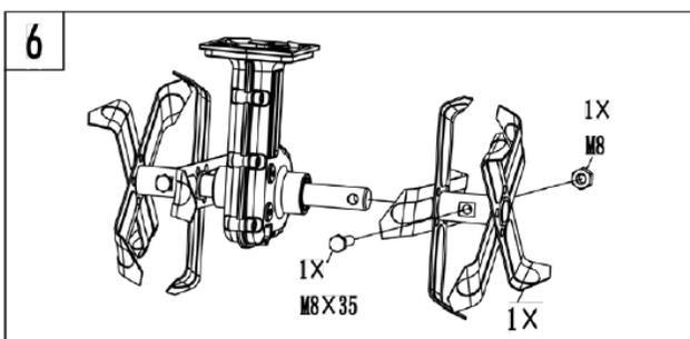
Replace worn or damaged parts with original replacement parts only. Parts from another tiller/cultivator may not fit properly causing an unsafe situation.
