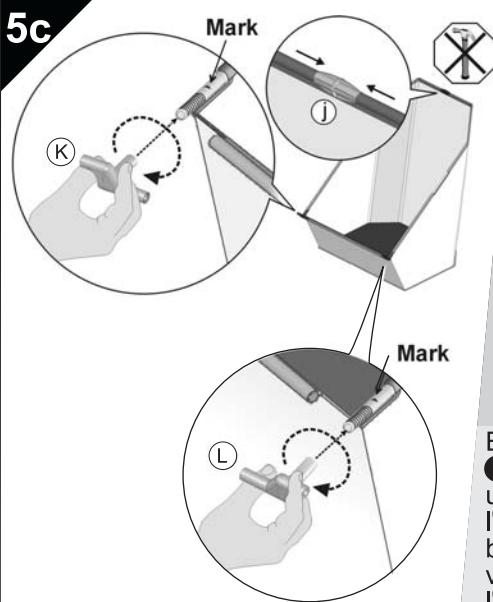
At top of the hopper bag, insert the smooth ends of the two rods **h** into the connector **j**. To connect the bottom left of the hopper bag, use connector **L** and screw the end with the single ring around it onto the threaded end until it meets the mark on the rod. Make sure the bent end of the connector is facing outward. Using connector **K** with two rings around one of its ends, repeat the same to connect the bottom right of the hopper bag.
