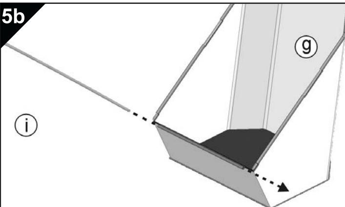
Insert straight rod **i** into sleeve on bottom edge of hopper bag **g**.
