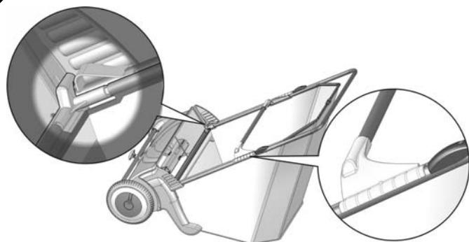
Position ends of the hopper bag connectors snug against the back side of the main sweeper body and snap the bag and frame into place mid way up the sides of sweeper handle.
