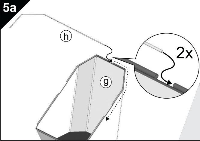
Starting with the threaded end, insert rod **h** into sleeve on top left edge of hopper bag **g**. Push rod all the way around until the end clears the sleeve on bottom left edge of the hopper bag. Repeat same for the right side.
