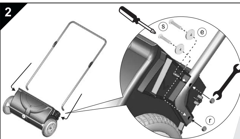
Insert screws **s** from the inside of the main sweeper body and through the bottom side of the handle. Then tighten nuts **r** on the outside to secure the handle in place
