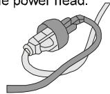
If using more than one extension cord, first tie the two cords in a knot as shown.
