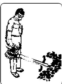
Hold the blower tube approximately 7 inches above the ground, switch your product on and using a sweeping motion from side to side, advance slowly. Keep the accumulated debris/leaves in front of you.
