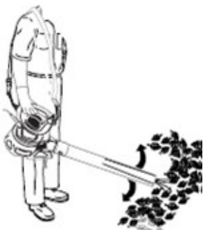
Once you have blown the debris/leaves into a pile, you can convert to vacuum mode to collect the debris.
