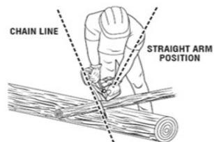
Allow the chain to cut for you; exert only light downward pressure. If you force the cut, damage to the bar, chain, or unit can result.
