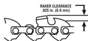
Every time the chain is filed, check the depth gauge clearance.
