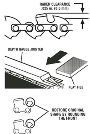
Depth gauges must be adjusted with the flat file in the same direction the adjoining cutter was filed with the round file. Use care not to contact cutter face with flat file when adjusting depth gauges.
