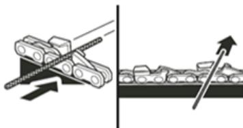
Lift file away from the steel on each return stroke.
