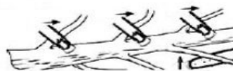
CUT LIMBS ONE AT A TIME AND LEAVE SUPPORT LIMBS UNDER TREE UNTIL LOG IS CUT FIG. 19
