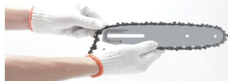
9. Hold the chain in position on the bar and place the loop around the sprocket. (Fig. 15)
