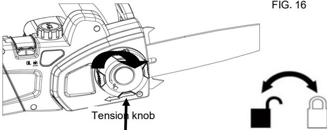
13. When the tension knob is fully tightened, the chain is the tightest. To minor adjust the chain tension, loosen the tension knob and turn it counter-clockwise slightly until the chain is correctly tensioned.
