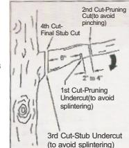
When pruning trees it is important not to make the finishing cut next to the main limb or trunk until you have cut off the limb further out to reduce the weight. This prevents stripping the bark from the main member.
