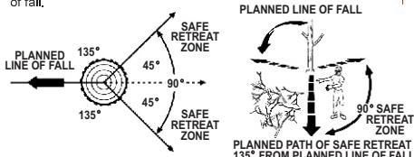
Before felling is started, consider the force and direction of the wind, the lean and balance of the tree, and the location of large limbs. These things influence the direction in which the tree will fall. Do not try to fell a tree along a line different from its natural line of fall.
