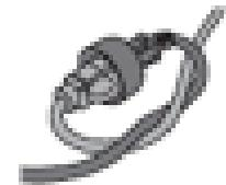
Use one of the plug-receptacle retaining straps or connectors described in this manual.
