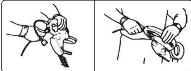
**1. WORKING POSITION**—Maintain proper footing and balance and do not overreach. Wear safety goggles, non-skid footwear and rubber gloves when trimming. Hold the tool firmly in both hands and turn the tool ON. Always hold the trimmer, as shown, with right hand on the switch handle and left hand on the front. Never hold the tool by the blade guard. Keep unit below waist level.
