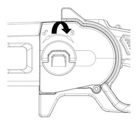
WARNING: The chain is not yet tensioned. Tensioning the chain as described under "TENSIONING CHAIN". The chain now needs to be inspected to make sure it is properly tensioned.
