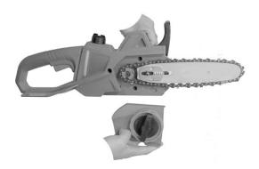
• Remove the bar and chain from the mounting surface.
