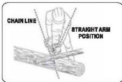
Squeeze the trigger and let the chain accelerate to full speed before entering the cut.
