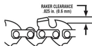
Use a flat file and a depth gauge jointer to lower all gauges uniformly. Depth gauge jointers are available in .020 in. to .035 in. (0.5 mm to 0.9 mm). Use a .025 in. (0.6 mm) depth gauge jointer. After lowering each depth gauge, restore original shape by rounding the front. Be careful not to damage adjoining drive links with the edge of the file.
