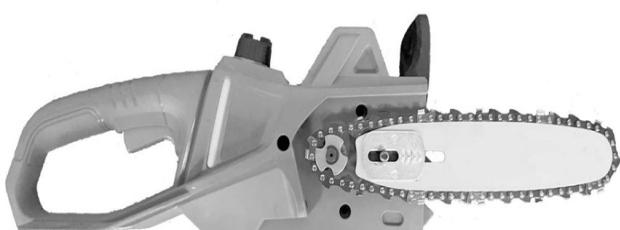
**NOTE:** If chain is too tight, it will not rotate. Loosen the knob slightly and turn the chain tensioner 1/4 turn counterclockwise. Lift the tip of the guide bar up and retighten the knob. Ensure that the chain will rotate without binding.
