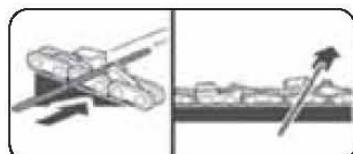
Lift file away from the steel on each return stroke.
