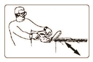
**4. SIDE-TRIMMING HEDGES—**Rotate handle to desired angle. Begin at the bottom and sweep up.
