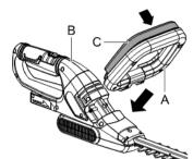
Secure the screws firmly on both sides of auxiliary handle.
