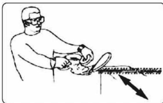
**4. SIDE-TRIMMING HEDGES—**Rotate handle to desired angle. Begin at the bottom and sweep up.
