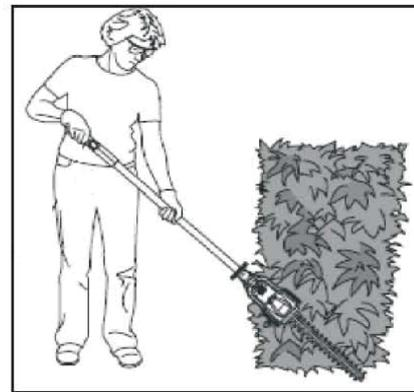
To use Pole Trimmer for trimming low-lying foliage or ground cover, hold the Pole Trimmer at the position as shown.
