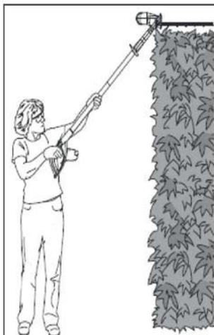
To use Pole Hedge Trimmer for trimming smaller hedges or shrubs, hold the Pole Trimmer at the positions as shown.
