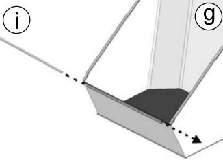
Insert straight rod **i** into sleeve on bottom edge of hopper bag **g**.
