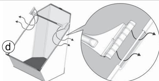
Align groove on the hopper handle **d** with the groove on the hopper frame rod **h**. Being careful not to bend the rod, push up from the bottom of the yellow edge of the handle and down on the rod at same time to snap the two together. Repeat for the other side.
