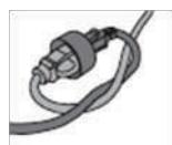
**DOUBLE INSULATION** – Double Insulation is a concept in safety in electric power tools, which eliminates the need for the usual three-wire grounded power cord. All exposed metal parts are isolated from the internal metal motor components with protecting insulation. Double insulated tools do not need to be grounded.
