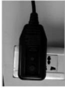
Plug GFCI into power receptacle. Press reset button; indicator should be "ON"; Press test button; indicator should be "OFF"; Press reset button for use. Do not use if test fails.
