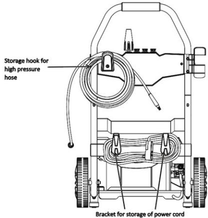
\* The bottom left bracket which helps secure the power cord may be rotated to the right to allow for easier removal of the cord.
