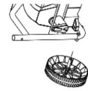
Insert the wheel axle through the hole on the lower washer frame. Secure the axle in place with the cotter pin provided.
