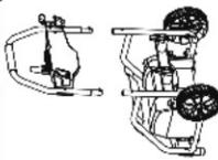
Insert the top handle into the lower handle while pressing on the button lock. Push the handle down firmly until the button lock snaps into place.
