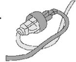
⚠ **WARNING:** Use outdoor extension cords marked SW-A, SOW-A, STW-A, STOW-A, SJW-A, SJTW-A, or SJTOWA. These cords are rated for outdoor use and reduce the risk of electric shock.
