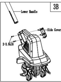
▲ WARNING: When connecting the tilling head and lower handle using the two self-tapping screws supplied, make sure the screws are securely tightened. Screw heads should be recessed below the surface. DO NOT START THE UNIT UNTIL TILLING HEAD AND LOWER HANDLE ARE SECURELY CONNECTED.
